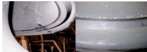
Figure 19: Seat ring and valve spindle show no dent marks after app. 1,000 hours.
