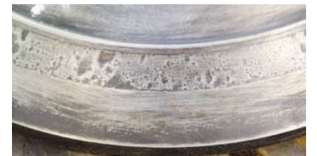
Figure 03: Typical dent marks of the seat of a valve spindle (MC60-type Nimonic after 8,300 hrs)
