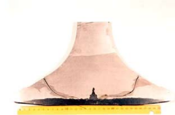
Figure 13: Macro cut through the center of a valve head (RTA62 Nimonic-type 6,430 hrs after repair)
