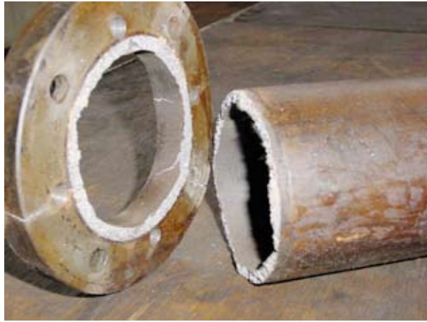
Figure 05: Low temperature corrosion of valve housing (MC-type 43,700 hrs)
