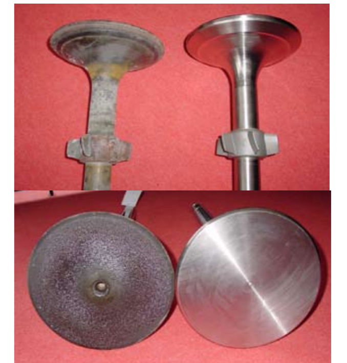
Figure 15 a/b: Nimalike spindle before and after remanufacturing
