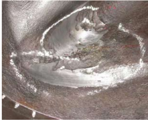
Figure 05: Low temperature corrosion of valve housing (MC-type 43,700 hrs)
