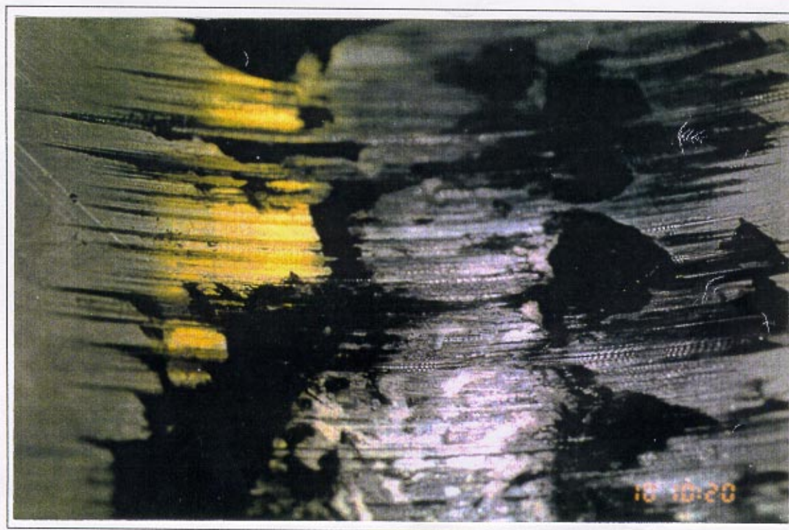
Fig. 2. Blackened and pitted bore
