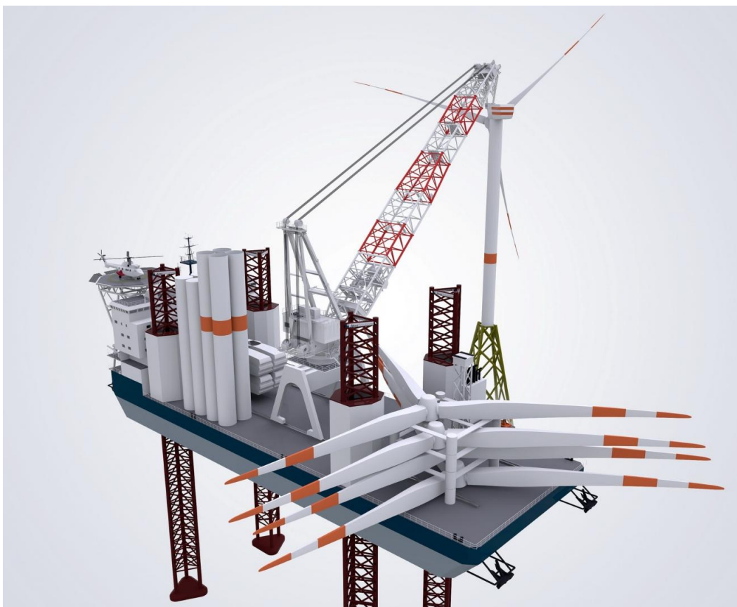
Picture Turbine Installation Vessel: Thanks to the optimized deck space around the 1000 ton offshore type gantry crane, three windmill foundations or five complete wind turbine assemblies of the 5 MW class can be stored on deck, thus increasing the installation efficiency.
