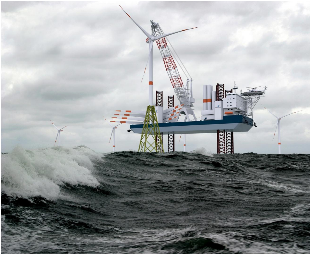
Picture Turbine Installation Vessel: This HPTIV can operate in year around weather conditions with an operational water depth range of 4.5 to 50 m.
