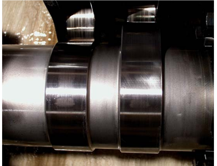
Fig. 27 Valve cams and roller guides for cyl. no. 6
