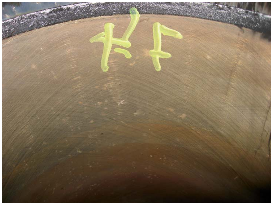
Fig. 10: Liner no. 3 exhaust side in the upper TDC point after 26,300 hrs of operation
