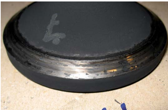
Fig. 13: Exhaust valve after 46,300 hrs of operation
