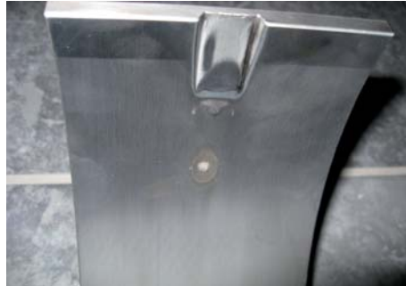
Fig. 21: Main bearing no. 2 - Cavitations mark visible
