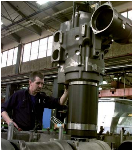
Fig. 28: L27/38 complete cylinder unit
