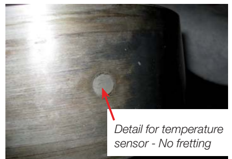
Fig. 20: Main bearing no. 1 - Back side of lower main bearing shell
