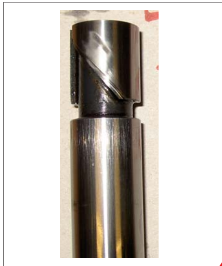
Fig. 23: Plunger with cavitation
