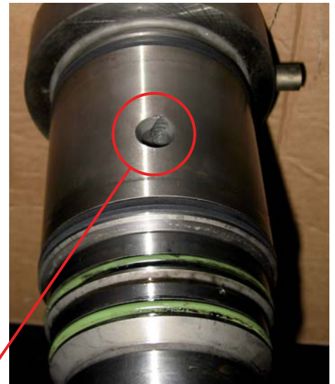
Fig. 24: Cavitation marks at the inlet bore low pressure side
