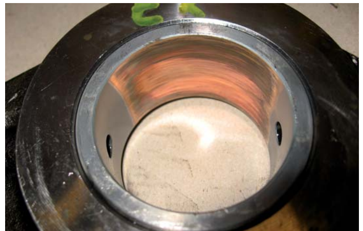
Fig. 14: Exhaust rocker arm bush after 46,300 hrs of operation. Can continue operation
