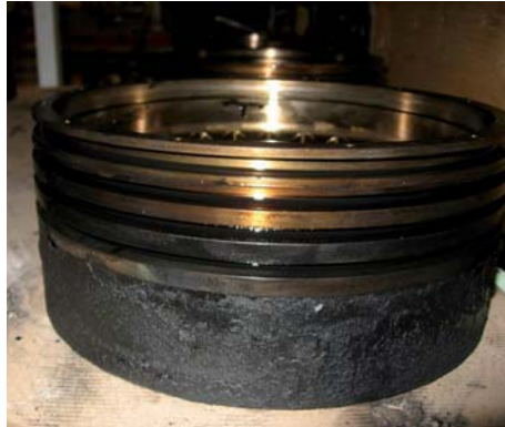
Fig. 15: Piston top crown in good condition after 26,300 hrs of operation since the last withdrawal
