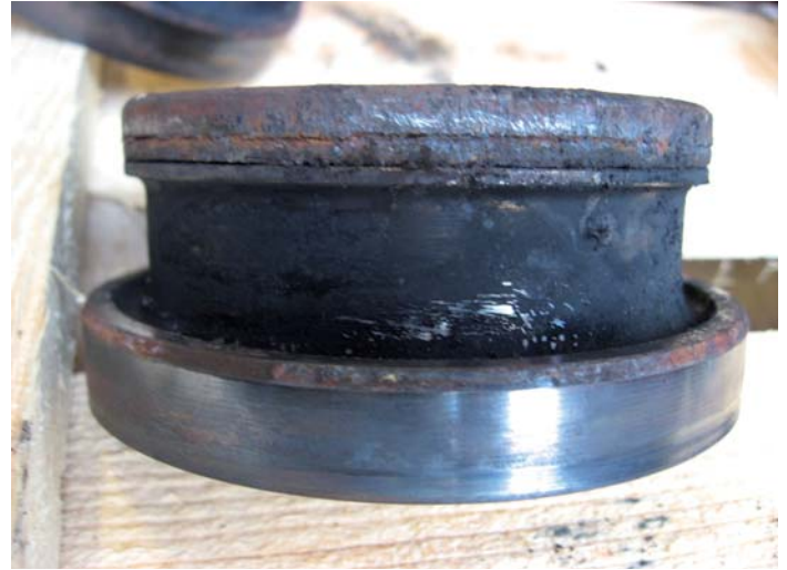
Fig. 12: Exhaust seat ring – corrosion-damaged due to inadequate cooling water inhibitor
