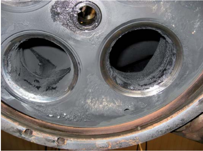
Fig. 11: Cylinder head inlet – and exhaust ring. Coke deposit limited after 26,300 hrs of operation
