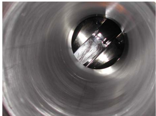
Fig. 12: Cylinder liner after the honing process
