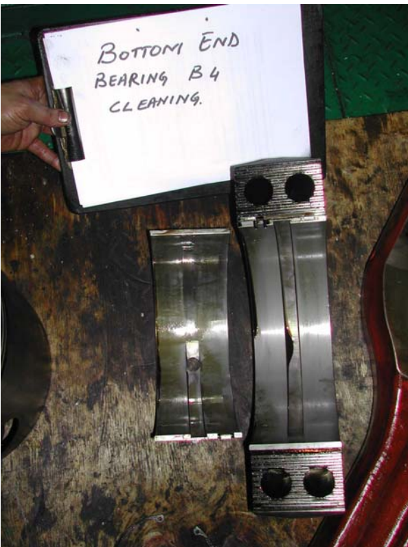
Fig. 15: Connecting rod bottom-end bearing dismantled and cleaned before dye checking.
