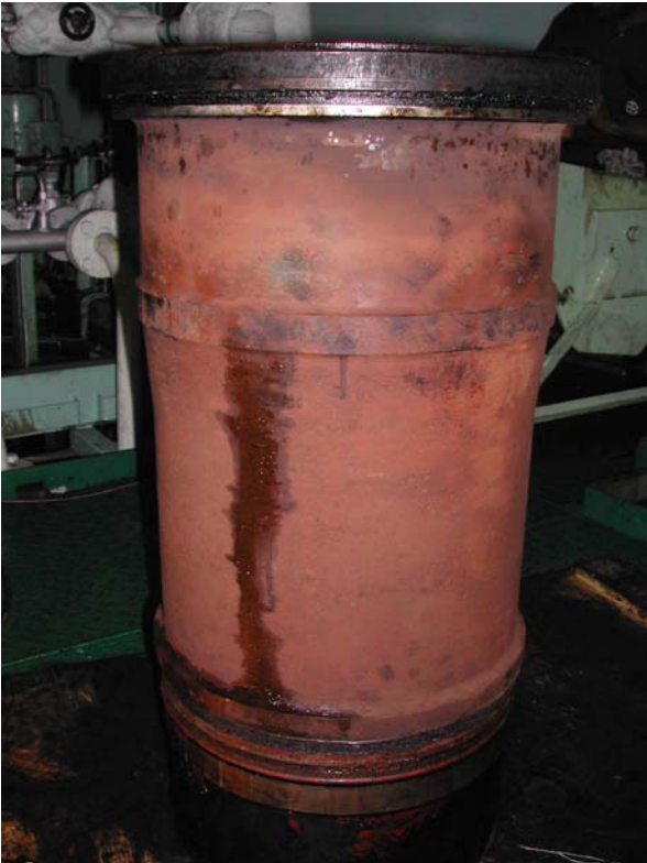
Fig. 10: Cooling water-side of cylinder liner. Cylinder liner O-rings for the cooling water spaces were renewed after inspection and cleaning
